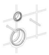
3. It is advisable to apply a small amount of lubricant (washing up liquid) to the flush pipe and pan connector to assist with fitting the toilet pan.
