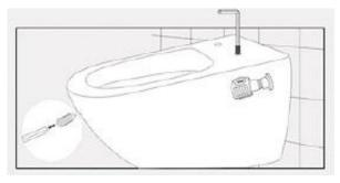
8. Once the installation is completed, a flush and leak test should be carried out and once it has been commissioned, the toilet can be sealed around the edge to finish.
